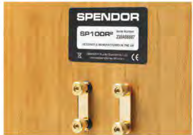
The S100R 2 has two pairs of binding posts compared to its predecessor’s three pairs.
