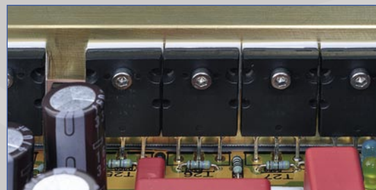
Power transistors with ceramic insulators and solid brass bar
